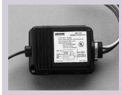
The MP Power Pack Series A can power up to three sensors. The internal relay can control up to 20 amps at either 120, 230 or 277, and 15 amps at 347 VAC ballast load.
